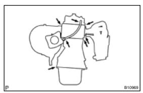
**6. INSPECT HOSES, CONNECTIONS AND GASKETS** Visually check for cracks, leaks or damage.
