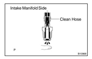
(b) Blow air into the intake manifold side, and check that it has a little difficulty for the air to pass through.
